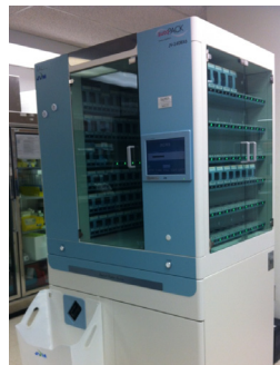
The new Auto-Pack Packager is a fully automated packaging system that supports bar-coding.
