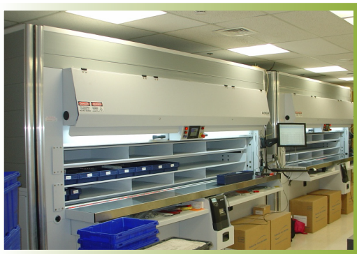
The new Carousel Cabinets take the place of the old "pick station" where medications were hand-picked.
